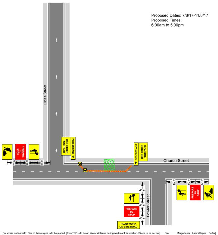
at start of works to notify pedestrians. Selection of sign is to comply with works on the day and space requirements. Pedestrian directional signs are also to be displayed for pedestrian guidance through the work site.
